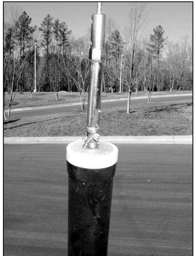
Fig 26 —Photo of the top of the loading coil. (Photo courtesy of Gary Pearce, KN4AQ.)
