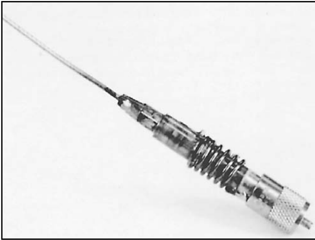
Fig 51—The 220-MHz \frac{5}{8} - \lambda mobile antenna. The coil turns are spaced over a distance of 1 inch, and the bottom end of the coil is soldered to the coax connector.
