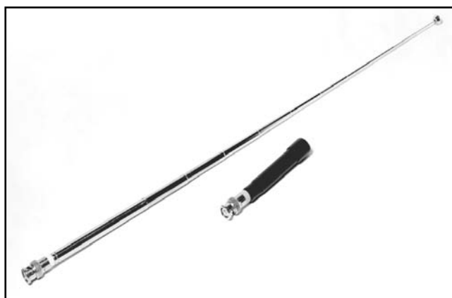
Fig 1 —Two mobile antennas—mobile because they may be used while in motion. Shown here are a telescoping \frac{1}{4}\lambda antenna and a “stubby” antenna, both designed for use at 144 MHz. The \frac{1}{4}\lambda antenna is 19 inch long, while the stubby antenna is only 3\frac{1}{2} inch long. (Both dimensions exclude the length of the BNC connectors. The stubby is a helically wound radiator.
