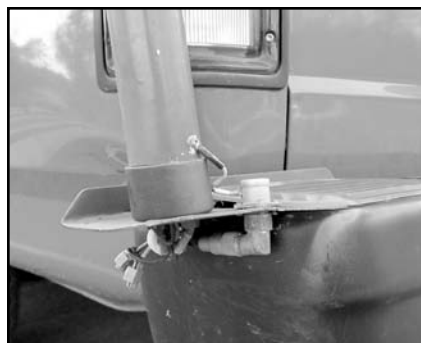
Fig 29—Base-mounting plate for Screw-driver installation on KO4TV's truck. Note the quick-disconnect dc motor connections and the SO-239 coax connector.
