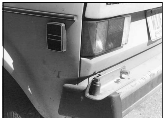
Fig 36—The mount for the mobile J is made from stainless-steel angle stock and secured to the bumper with stainless-steel hardware. Note the \frac{1}{2} -inch pipe plug and a PL-259 (with a copper disc soldered in its unthreaded end). These protect the mount and connector threads when the antenna is not in use.
