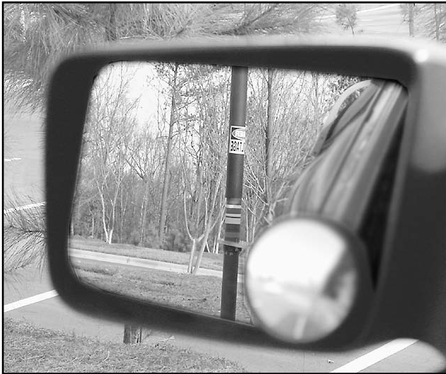
Fig 34—Remote control by the rear-view mirror—tuning by the stripes! (Photo courtesy of Gary Pearce, KN4AQ.)
