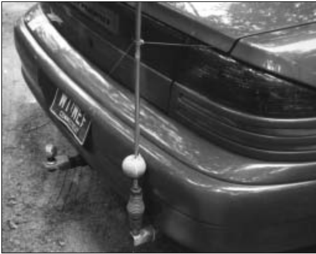
Fig 2—A typical bumper-mounted HF mobile antenna, as used by W1WEF. Note the nylon guy lines and the tennis ball used as a shock absorber. (Photo courtesy W1WEF.)
