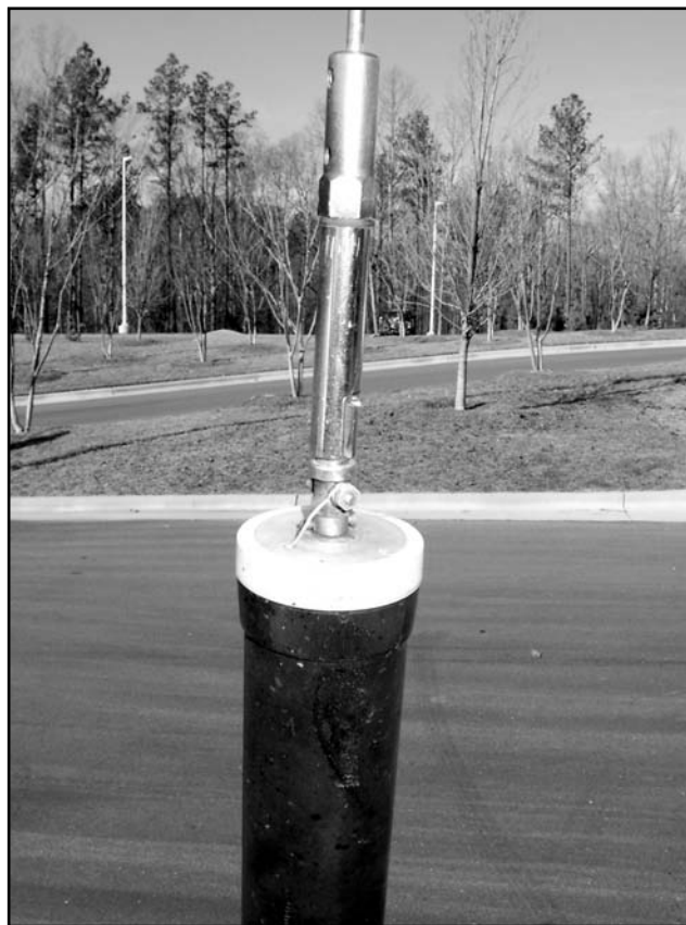
Fig 26 —Photo of the top of the loading coil. (Photo courtesy of Gary Pearce, KN4AQ.)
